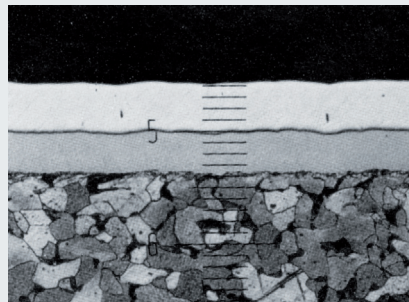
Illustration of a KANICHROM® layer on steel at 150 times magnification.
